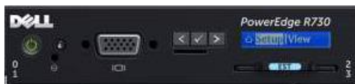
Figure 9. R730 LCD control panel
